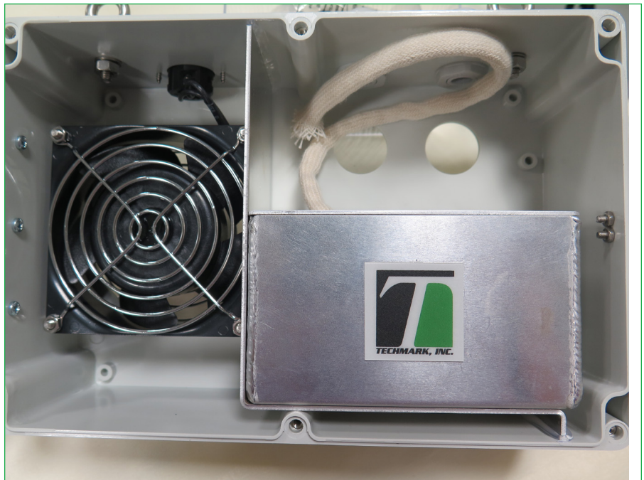
New aluminum reservoir replaces plastic units.
