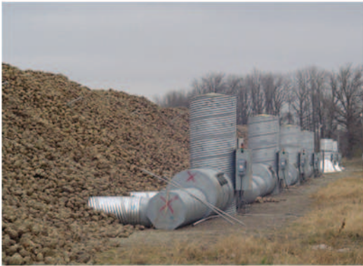
ventilation towers on a sugarbeet pile
